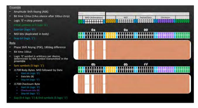
The SSC P485 bidirectionally converts between J1708 and J2497. If it observes activity on the J1708 bus while the J2497 is idle, it sends a preamble followed by the body; likewise, when activity is observed on the J2497 bus, a J1708 message is sent. For example, when a LAMP ON message is observed on the J2497 bus, the SSC P485 converts it to J1708, like so:
