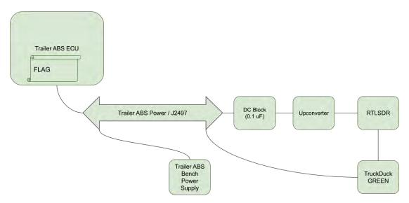
In this challenge we gave competitors access to the J2497 powerline interface of a trailer brake controller via both an SDR (for read) and a bit-banged GPIO on a TruckDuck/BeagleBoneBlack (for write). There are a bunch of different ways to slice this, but in general you will need to solve the following for your bench setup:
