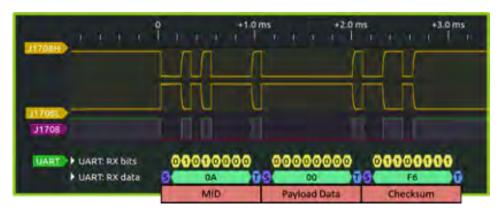
The alternative transport realized by the Intellon SSC P485 is that of a translation between the RS-485 physical layer and powerlines, but the first byte (the MID in J1708) plays an important role in arbitration for the bus.
