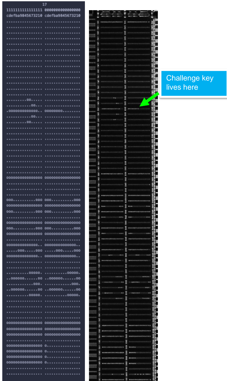
Figure 23. ASCII art rendering of bit plane 17 (left) and FIB image of bit plane 21 (right) from test device.
