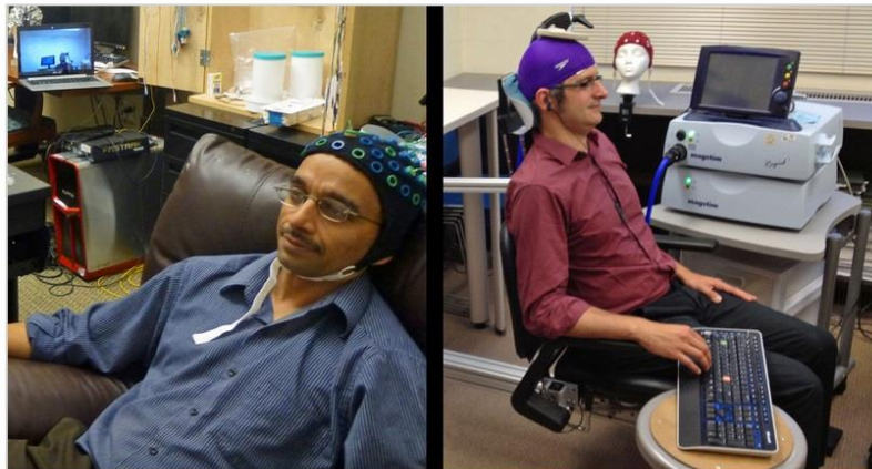
University of Washington researcher Rajesh Rao, left, plays a computer game with his mind. Across campus, researcher Andrea Stocco, right, wears a magnetic stimulation coil over the left motor cortex region of his brain. Stocco's right index finger moved involuntarily to hit the "fire" button as part of the first human brain-to-brain interface demonstration. (Credit: University of Washington)
