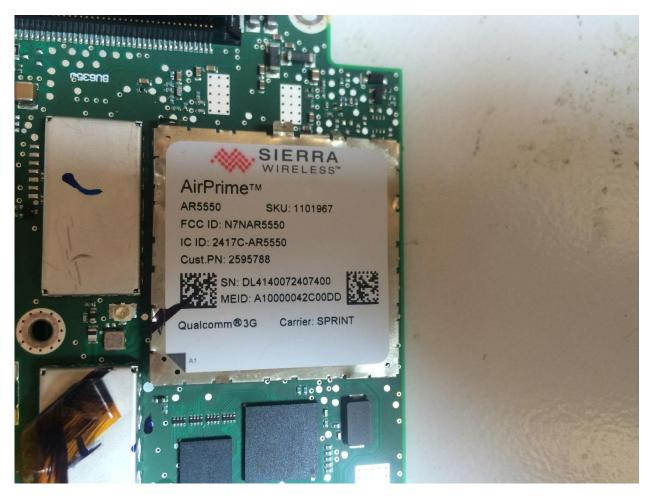
Figure 16: Sierra Wireless AirPrime AR5550 from a Harman Uconnect system
