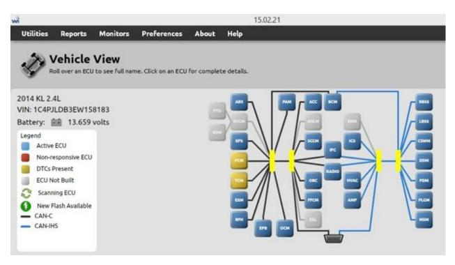
Figure 46: 2014 Jeep Cherokee ECU diagram from the WiTech software
