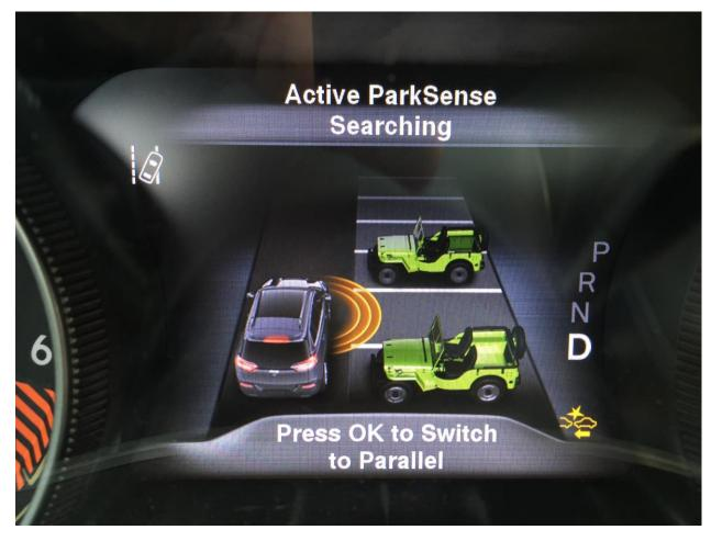
Figure 5: Display while using PAM system
