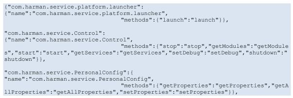
Examining and categorizing all the D-Bus services and method calls over TCP is an exercise left up to the reader, but we've found several that permit direct interaction with the head unit, such as adjusting the volume of the radio, accessing PPS data, and others that provide lower levels of access.
