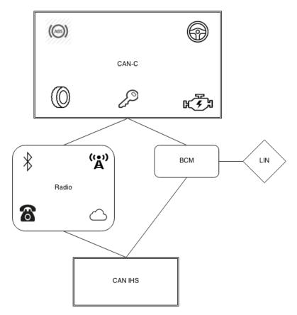
Figure 2: 2014 Jeep Cherokee architecture diagram
