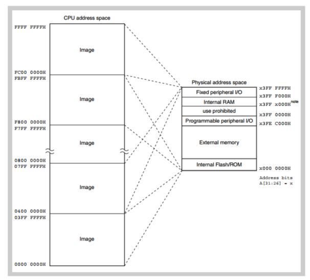
The 64 MB physical address space is seen as 64 images in the 4 GB CPU address space:
